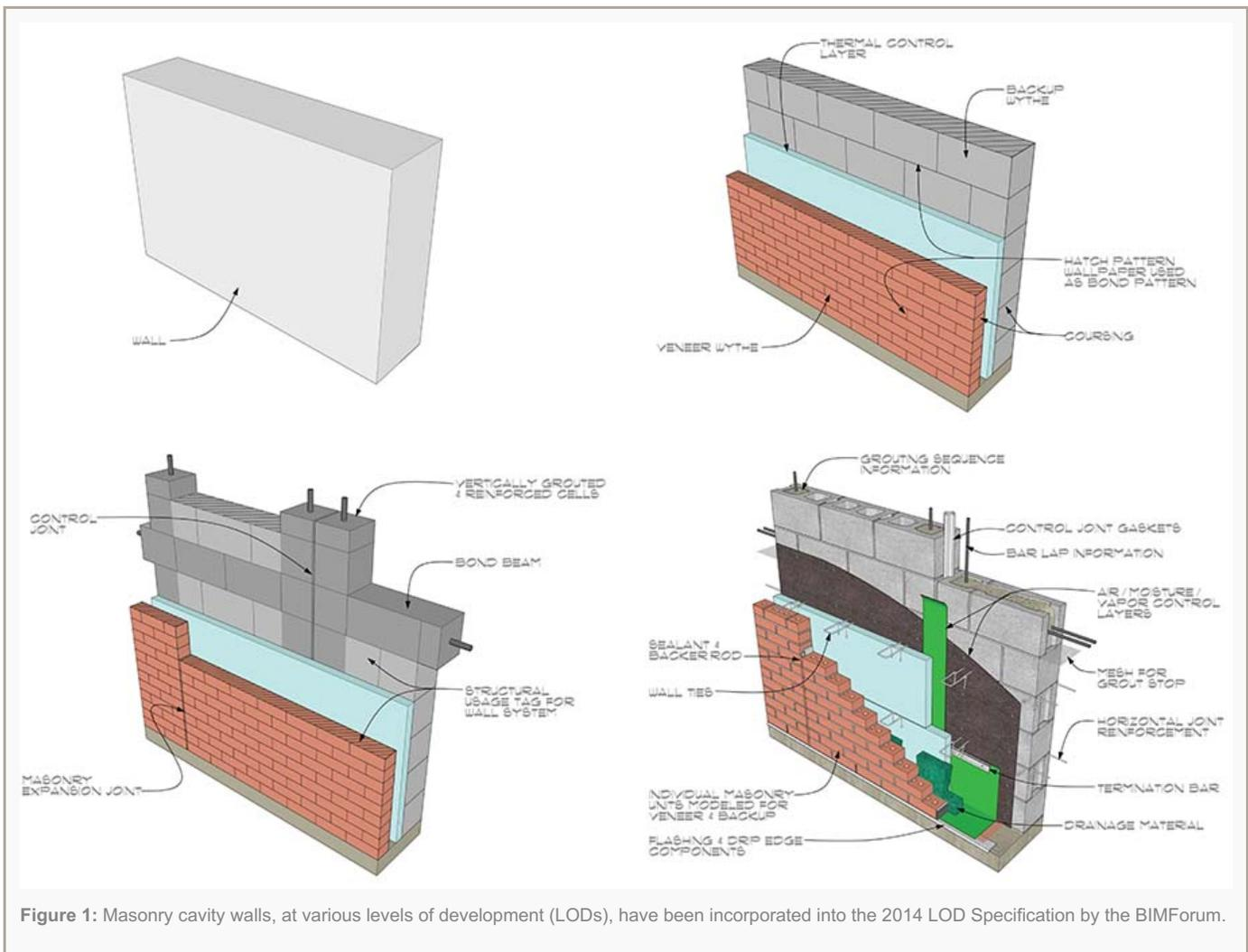
Figure 1: Masonry cavity walls, at various levels of development (LODs), have been incorporated into the 2014 LOD Specification by the BIMForum.
